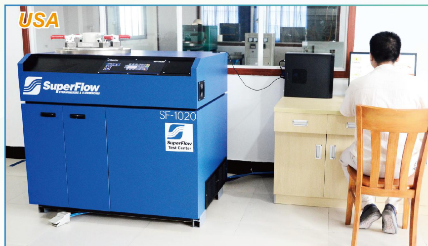
Back Pressure Drop Test Equipment 背压测试仪
