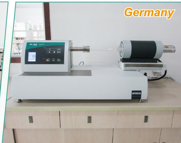
Coefficient of Thermal Expansion Test Equipment 热膨胀系数测试仪
