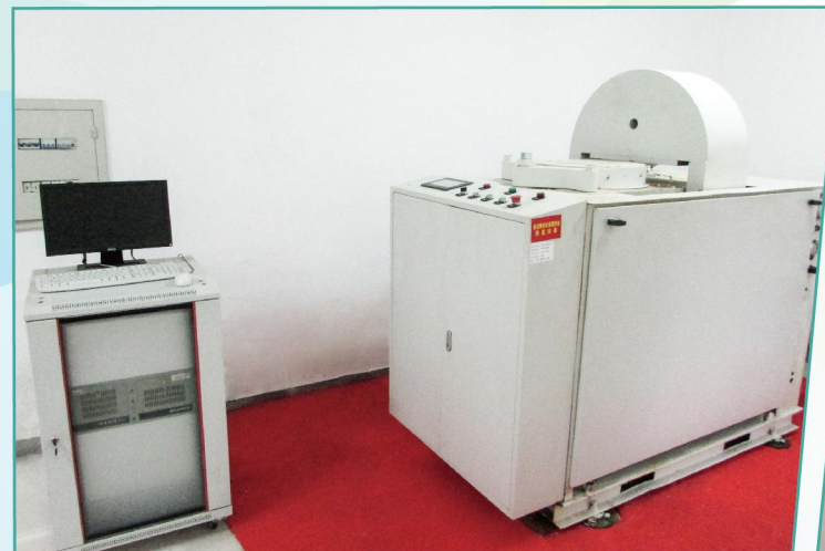
ISO Strength Test Equipment 等静压强度测试仪
